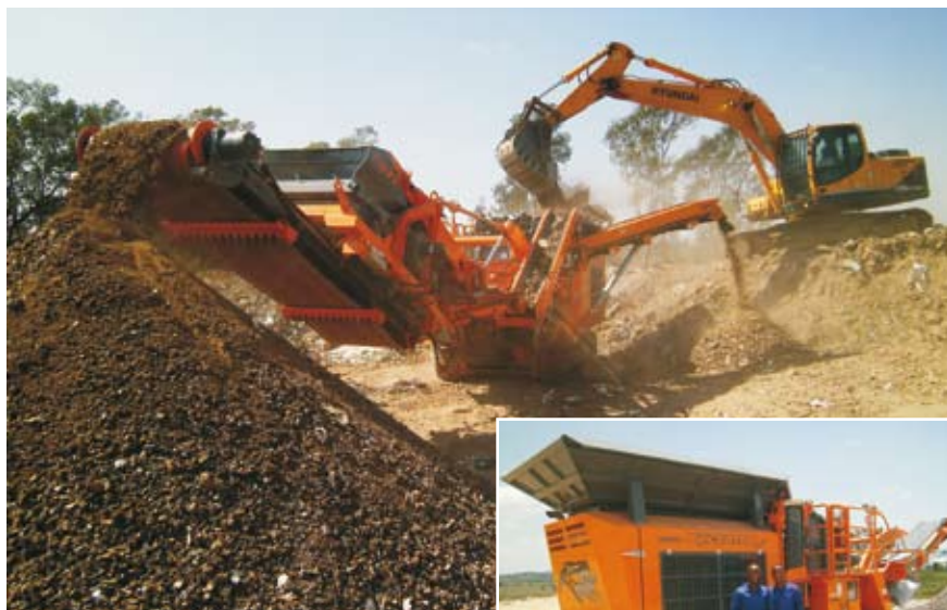
Rockster R700S at a landfill in Johannesburg, using the return belt as a stockpile conveyor
