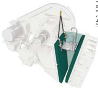
Metso Nordberg C-Series jaw crusher's maintenance platform
