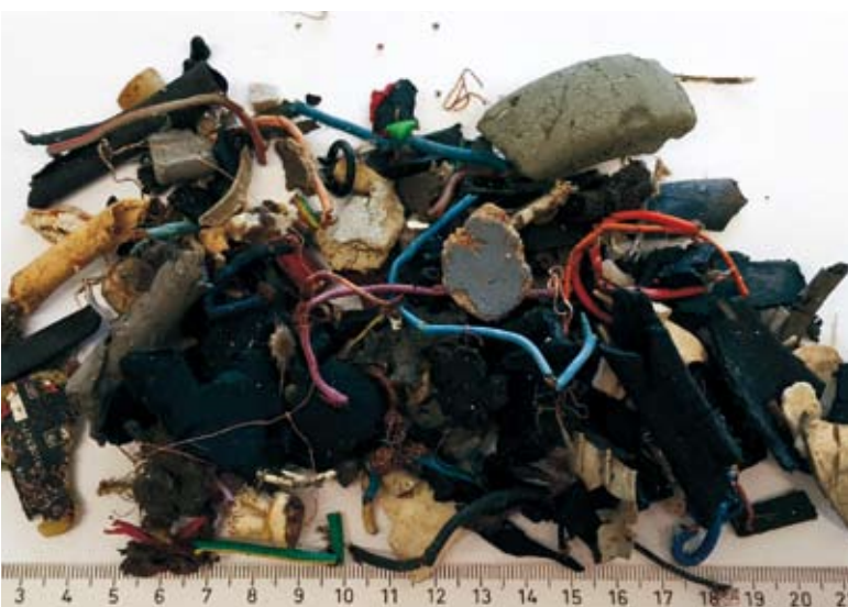
ASR is a mix of cables, hair wires, plugs, connectors, PCB, plastic and organic residue
