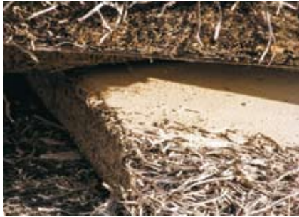
Medium density fiberboard (MDF) is an engineered wood panel product composed of refined virgin wood fibers, mixed with resin and wax and pressed into flat sheets under pressure and at elevated temperature
