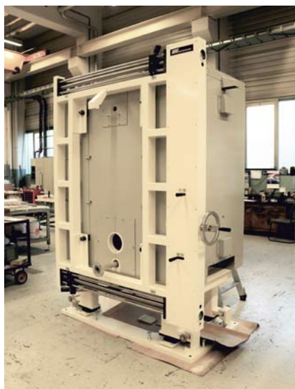
Melt filter for recycling PET flakes: NSF38
