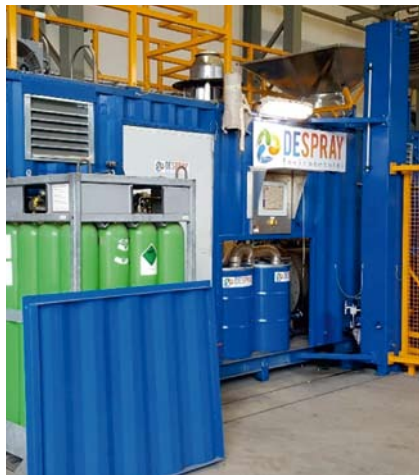
DeSpray DS1500, capable of processing 1500-2000 cans per hour
