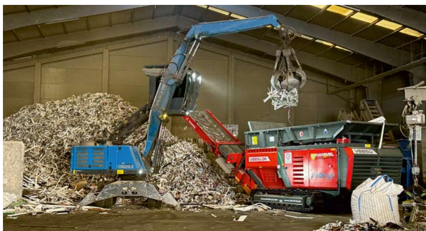
HAMMEL pre-shredder VB 850 DK – processing of aluminium
