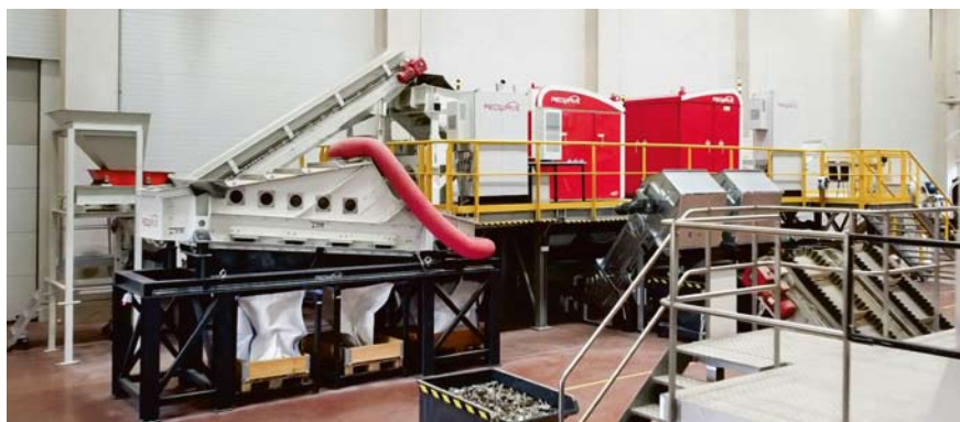
REDWAVE XRF with spectral analysis
