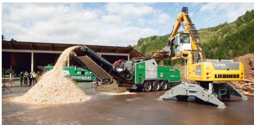
The high-speed Axtor universal chipper is one of the most flexible machines for processing wood and green cuttings
