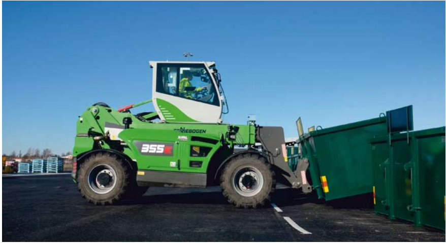
The 355 E impresses with a stacking height of 8.5 metres
