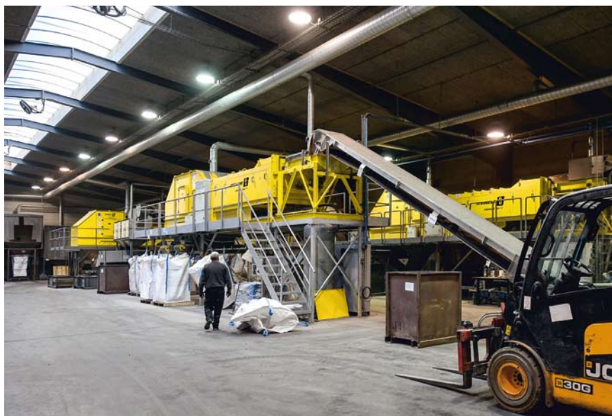
A STEINERT XSS T EVO 5.0 at Scanmetals produces ultra-pure aluminum. Heavy metals are sorted out
