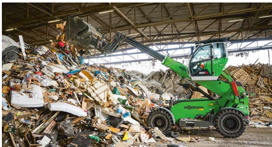
The elevating multicab of the 360 G offers the driver a 360° panoramic view
