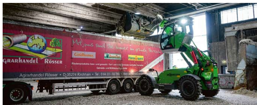
The telescopic arm of the Sennebogen 360 G reaches deep into the truck to load secondary fuels efficiently and evenly
