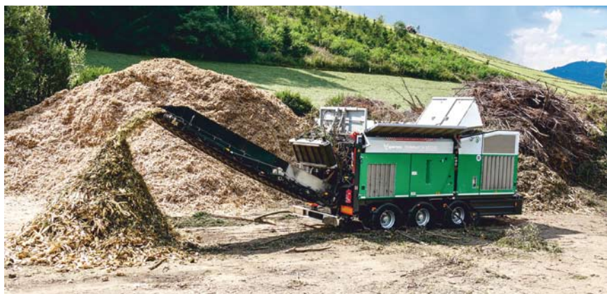
The efficient shredding of a wide variety of materials, from household and commercial waste to tyres to washing machines, is no problem for the stationary or mobile Terminator
