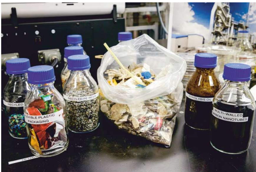
Different types of plastics, including marine waste litter in the middle, that can be turned into hydrogen and carbon nanotubes using NTU Singapore’s pilot plant
