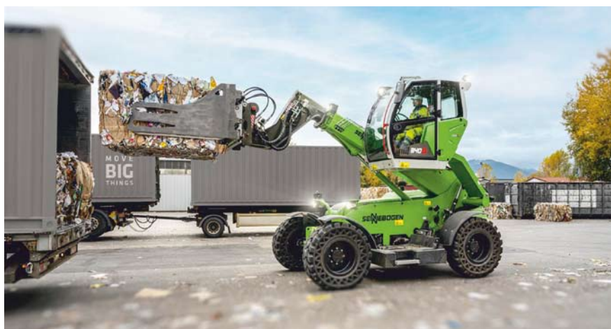
The viewing height of up to 4.10 m allows the operator optimal visibility in the loading process
