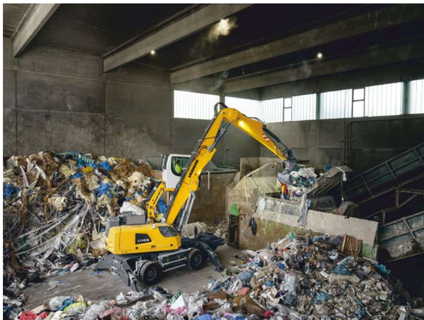
The LH 26 M Industry E at Bauma 2022: The wired electric material handler is equipped with a battery-operated Mobility Kit for temporary operation independent of the mains
