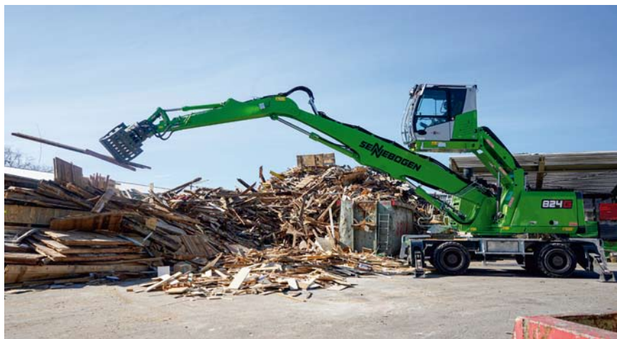
The sorting grab places the wooden spades in the designated position
