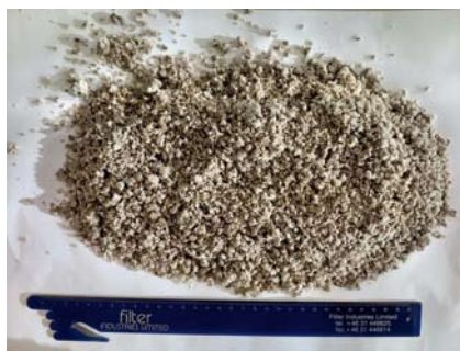
This is the powdered SiGS slag that can act as a substitute for cement in concrete
