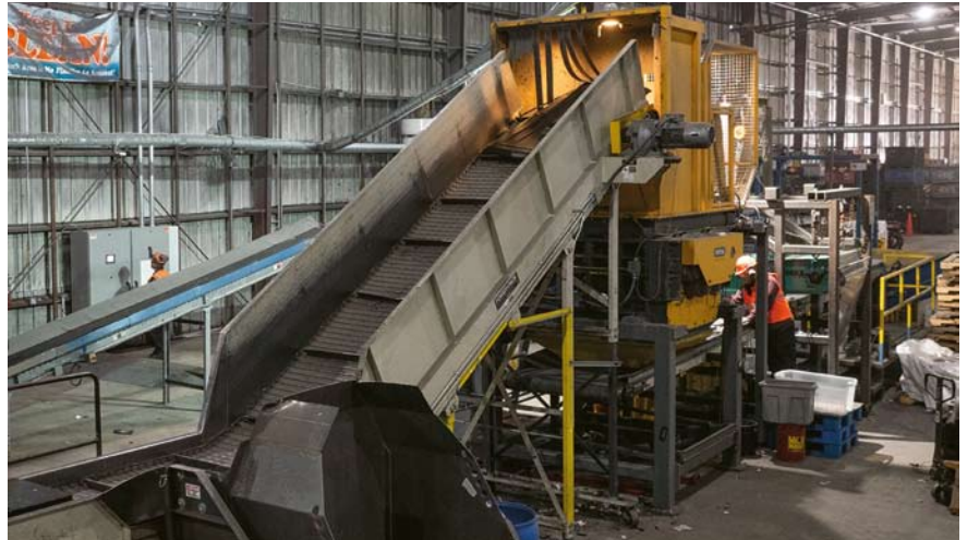
The RS100 shreds up to 12 tons/day and is part of a comprehensive recycling plant
