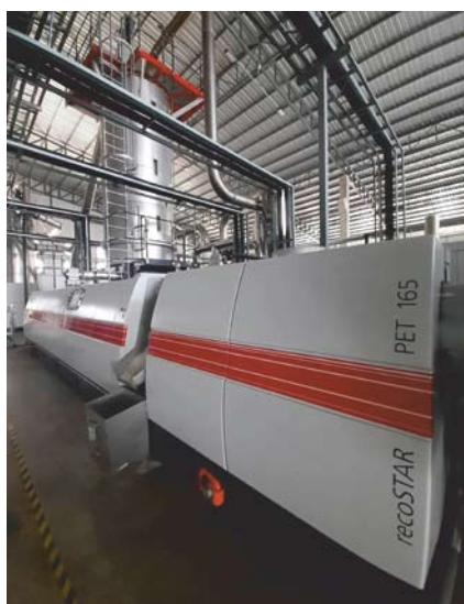
The Starlinger bottle-to-bottle recycling line installed at Royce’s production site in Sam Phran, Thailand
