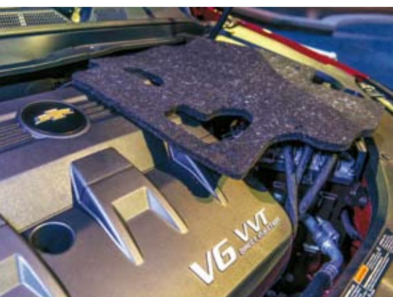
The Chevrolet Equinox V6 engine cover, set on top of the engine as a demonstration, includes water bottles collected from five GM facilities
